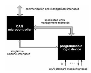
Figure 2 CANELy Hardware Architecture
